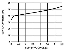
FIGURE 3. SUPPLY CURRENT vs SUPPLY VOLTAGE
