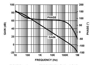
FIGURE 7. A<sub>VOL</sub> vs FREQUENCY @  $1k\Omega$  LOAD
