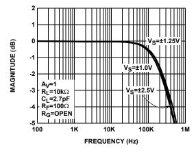
FIGURE 1. FREQUENCY RESPONSE vs SUPPLY VOLTAGE
