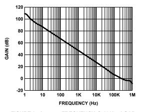
FIGURE 8. A<sub>VOL</sub> vs FREQUENCY @  $100k\Omega$  LOAD
