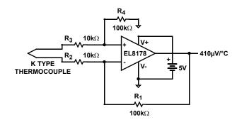
FIGURE 12. THERMOCOUPLE AMPLIFIER
